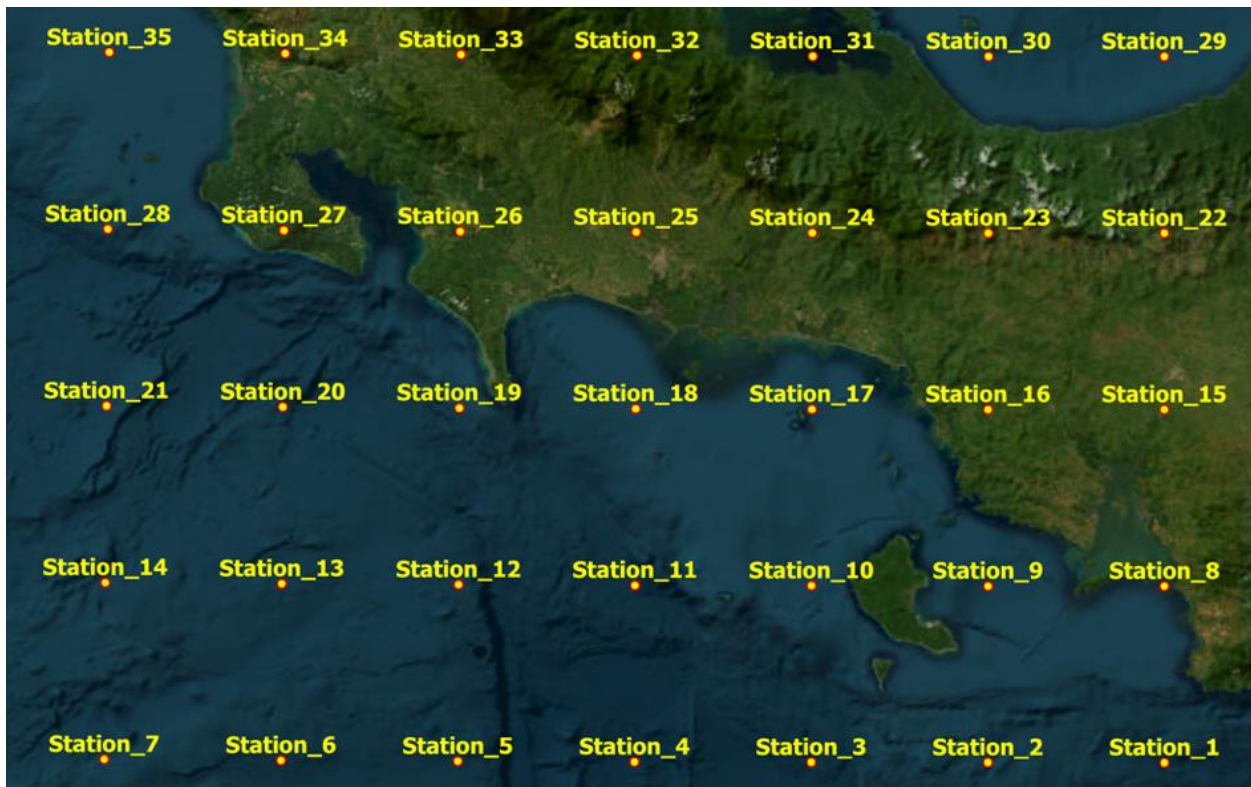
Figure 4-2: ERA5 Hindcast Stations for Wind and Wave Parameters Offshore of Puerto Armuelles. Station Numbering is Arbitrary.
